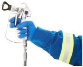
process involves the atomizing of the adhesive, during which the substance is converted into small droplets. The atomized adhesive drops, when sprayed, are airborne between the spray mechanism and the
