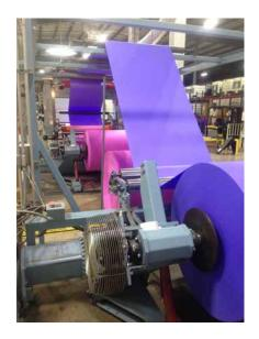
In addition to protective barriers, laminations can also impede the transmission of light. Different light barrier coatings are applied to products such as playing and trading cards and various double-sided advertisements; these coatings can also be applied to solar energy products. The popularity of these applications has encouraged manufacturers to rely on web lamination, which can improve the protective qualities and overall aesthetics of the substrates used.
